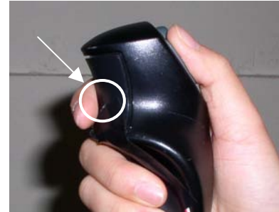
Figure 6. Force-sensing resistor's attached on 3D spatial mouse
